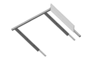
Attaching the shuttering skin to H20 Beams with nails or screw nails .The H20 beams offer a firm base for
