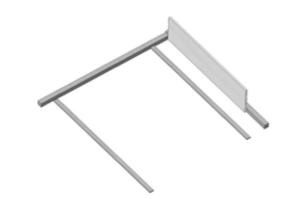
Positioning the H20 beams in their positions  $\ensuremath{\mathfrak{E}}$ attaching the H20 beam to steel waller with the
